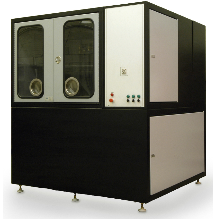
Typical Pressure Flushing Rig
