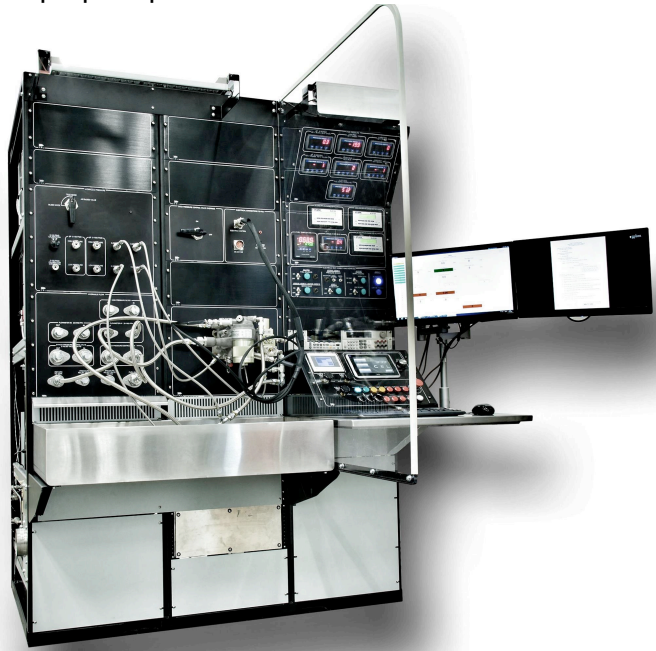
Typical Fuel Control Unit Test Stand with DAS under test
